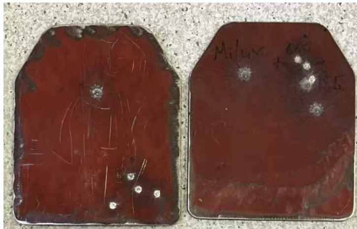
*Left: 5 hits of 5.45x39 7n10 (common to AK-74), Right: 5 hits of 7.62x54 LPS (common to Dragunov rifle and PKM machine gun)*
